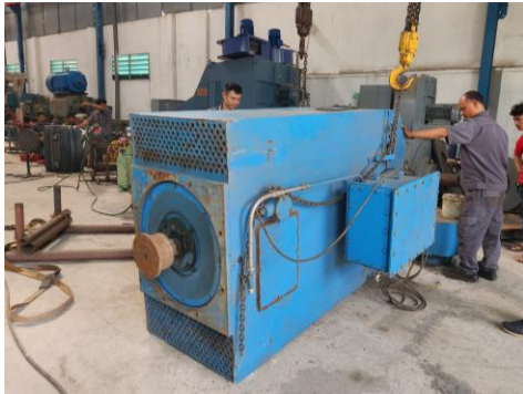
Service of Overhaul of Lift Pump Motor 6,6kV, 344kW for Offshore Platform
