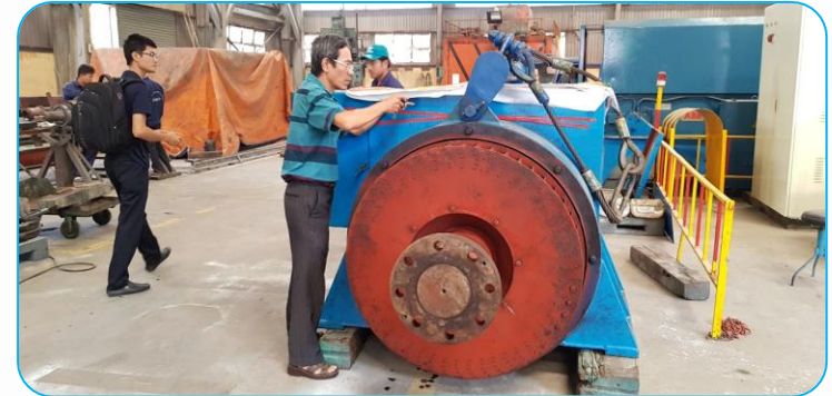
Service of Overhaul of Alternator 2,2 MW for Offshore Platform
