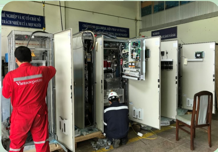
UPS System 30kVA for Offshore - Vietsovpetro
