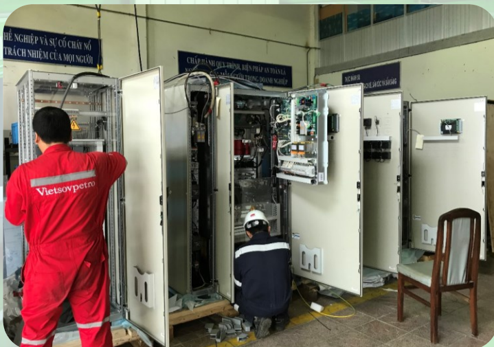
UPS System 30kVA for Offshore - Vietsovpetro
